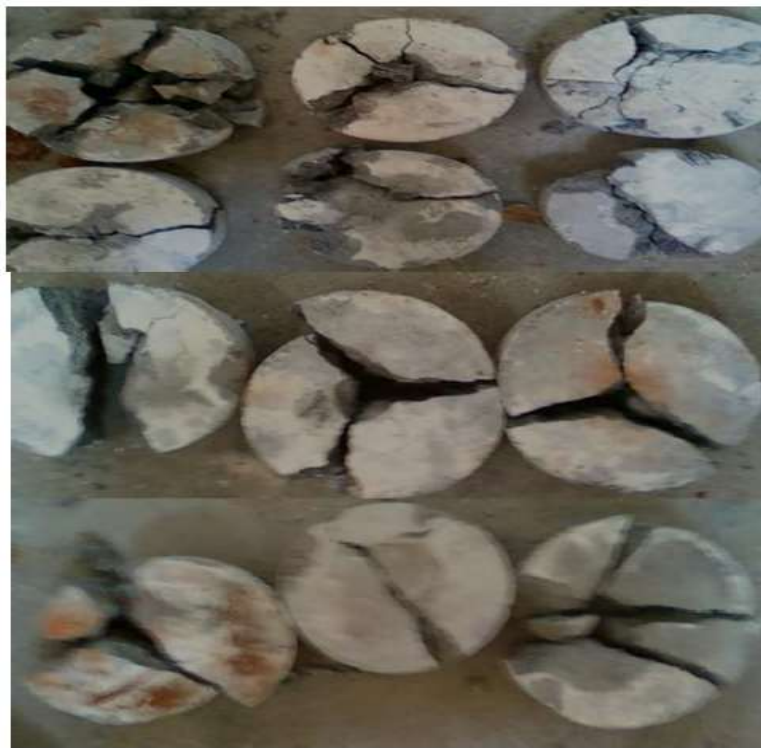
Figure 3.4 Failure Pattern of R3, R2, R1 & R0 Specimen
