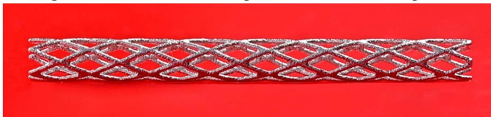
Figure 3. 3D Printed SS 316L powder stent with SLM process
