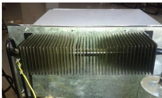
Fig. 6 Natural Air Cooled Condenser
