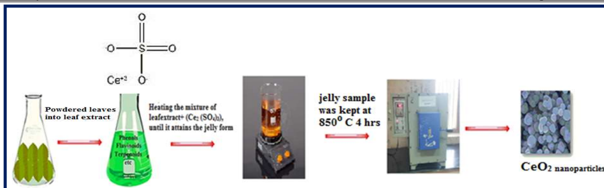
Fig. 1 Procedure for preparation of Piper betel L. leaf mediated CeO 2 nanoparticles
