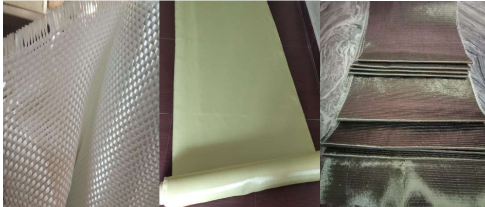
Fig. 1 - FRP laminates (a) GFRP; (b) AFRP; (c) BFRP
