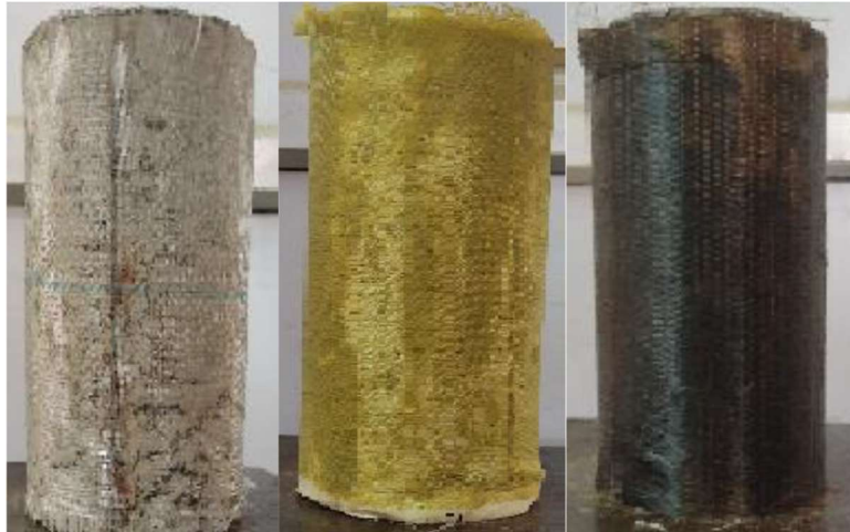
Fig. 5 – FRP wrapped specimens
