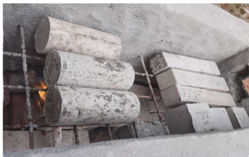
Fig. 3 – Fire exposure on concrete specimens
