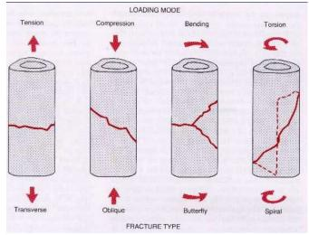
Fig 1. Fracture Mechanics
