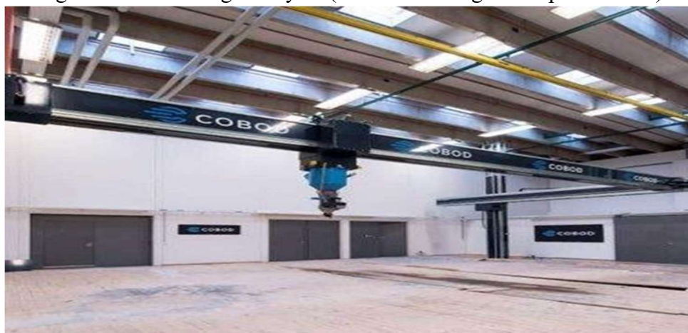
Figure 4: COBOD BOD2 3D House Printer - Gantry Type; Developed by Printheus Company, Denmark
