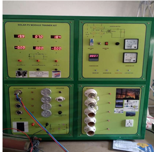
Fig.9 Solar PV Trainer Module with various DC loads.
