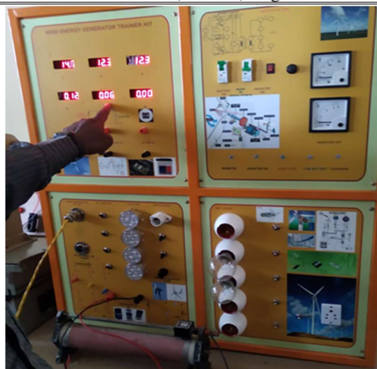
Fig.8 Wind Generator Module with Variable resistive load and AC loads.
