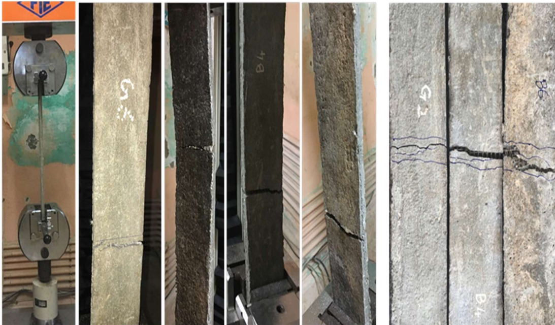
Figure 7. Failure of TRM tensile specimens.
