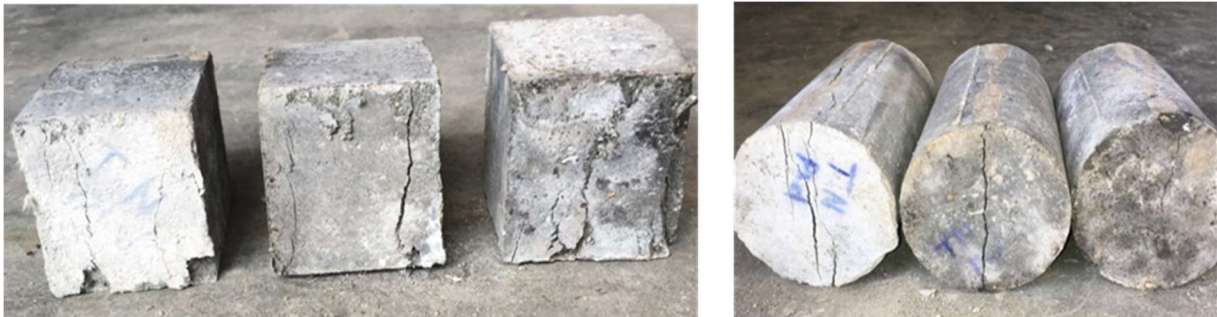
Figure 1. Failure of (a) mortar cubes, (b) mortar cylinder
