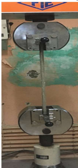
Figure 5. Uniaxial tensile test set-up.
