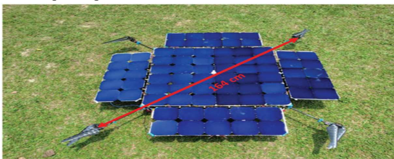
Figure 3: Photo of the solar quadcopter with 5S solar modules [27]
