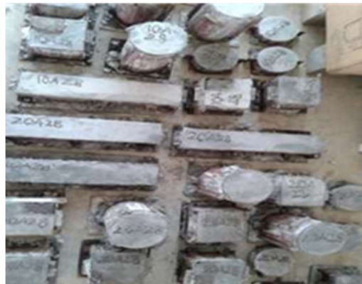
Fig. 1 Casting of Specimens
