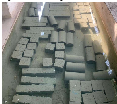
Figure 6- Curing of moulds
