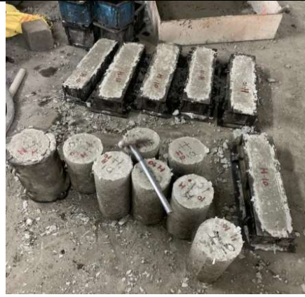
Figure 4- Cylinder and beam mould
