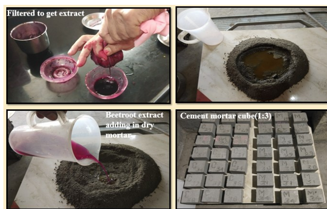
Figure 1 Mixing of beetroot extract (self-curing agent) in a dry mortar (1:3)
